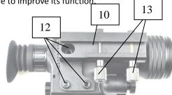
riflescope for an extended period of time, put a small drop of Loctite 242 (Blue) on the screws' threads prior to attaching the mount to the monocular. This will prevent the screws from becoming loose over time. **Do not use Loctite Red or similar permanent solutions!**
